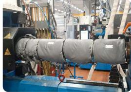
Insulating sleeves on an injection press at Texen CMSI
